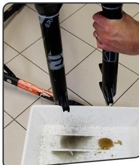
Place an oil recovery tank under the fork vertical line. Gently extract the lowers, oil will spill down on the recovery tank.
