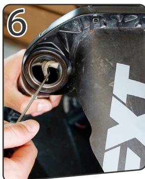
Using a pick-up tool remove the internal foams.
