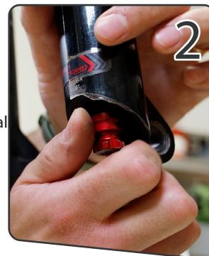
Remove the rebound knob by firmly pulling it (small rotatory movements may facilitate the operation)
