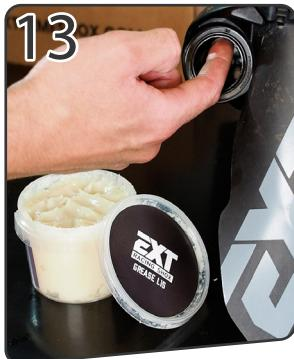
Put a small amount of EXT L1S grease inside the scrapers, do not exceed, a small film of lubricant is sufficient.
