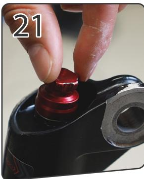
Push back in position the red rebound adjustment knob. To check the correct fitment make a complete adjustment turn.
