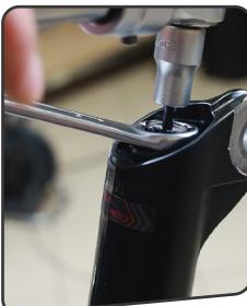
Assembly back in position both the knobs that has already been carefully cleaned. UNSCREW (turn counter-clockwise) at 8Nm using a torque wrench.
