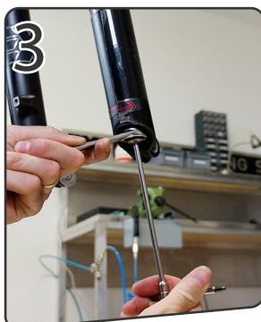
Using a 19mm spanner unscrew half a turn the external nut to break the Loctite. Now start SCREWING (turn clockwise) the central pin with a 4mm allen key
