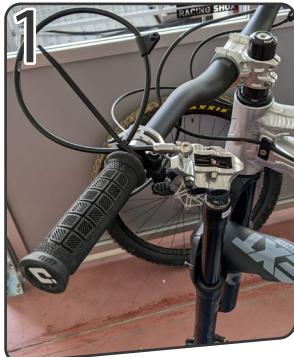
Place the bike on the stand and remove the front wheel. Remove the front brake caliper (also the tube holder) and fix it (as for example with a cable tie) to the handlebar in order to protect it from any oil spurt.
