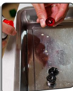
Carefully clean the lower knobs from old Loctite.
